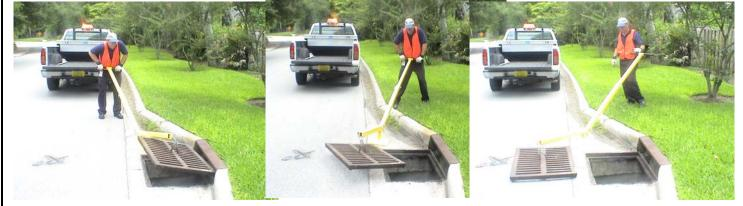
1. Position the Ultra-GrateLifter on a stable and level surface adjacent to the grate. Attach the grate hooks in the center of the grate.
