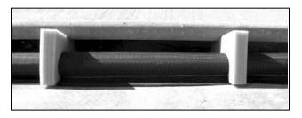
Note: The top of each Anchoring Wedge is perforated. If the Wedge is too large for the inlet, simply tear off the top section and reinstall (a second perforation is available if needed). The front of the Anchoring Wedges should be flush with the face of the inlet.
